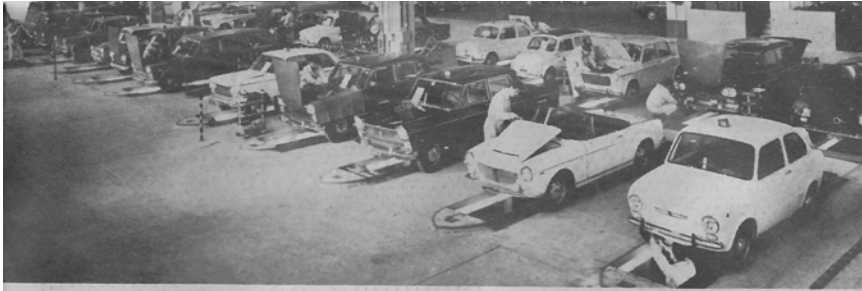
GREASE PITS seem to be individual, primitive forerunners of hydraulic lifts, but take a look underneath >
